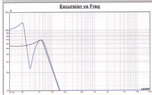
Figure 13: Cone excursion curves for the 14/13.5-V curves in Figure 11
