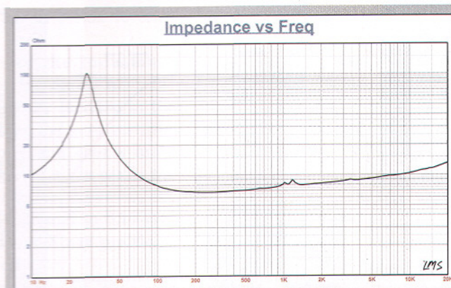
Figure 10: SB Acoustics MW16R woofer free-air impedance plot
